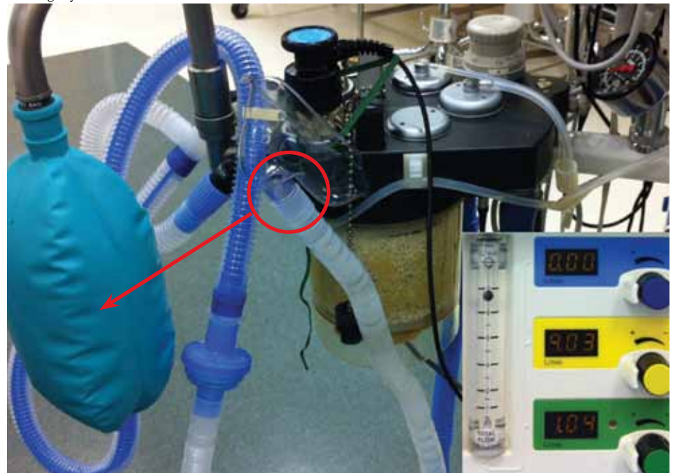
Figure 2: Aerosol Oxygen Mask (or regular oxygen face mask with thin diameter tubing removed) Attached to Circle System.
